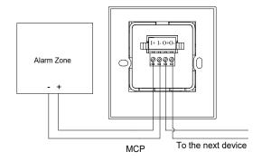
Note: The call point cannot be directly connected to 24VDC power, or its internal components may be damaged. It must be connected to a compatible power limited fire alarm control panel (28VDC/60mA max.).
