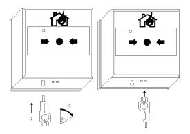
A test tool is provided as spare part. The test tool is used to keep continuity during commissioning or maintenance when MCP is not installed, so that cable test can be carried out easily and make the circuit completed.
